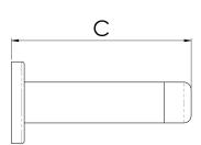
A slimline and elegant skirting or wall mounted door stop on a rose feature. The base rose unscrews allowing it to be fixed to the wall or skirting board, the door stop main body is then screwed back on for neat concealed fix. Screw supplied.
