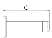
A slimline and elegant skirting or wall mounted door stop on a rose feature. The base rose unscrews allowing it to be fixed to the wall or skirting board, the door stop main body is then screwed back on for neat concealed fix. Screw supplied.
