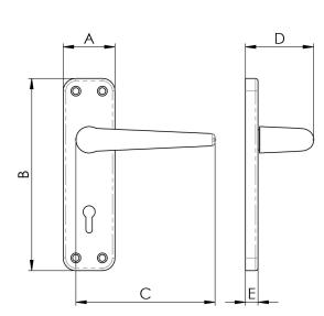
Contract Lever on Backplate. A slender straight lever tapering slightly towards the end on a rectangular face fix backplate allowing easy and quick installation. Ideal contact specification. Comes with a 10 year mechanical guarantee and is Fire door rated.
