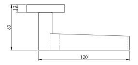
Lever on a concealed fix 2 part screw on round rose. A rounded straight lever, simple but elegant, ideal for creating a minimalistic effect. Ergonomic and comfortable to use, ideal for heavy use in the office or school. Comes with a 25 year mechanical guarantee and is Fire door rated.
