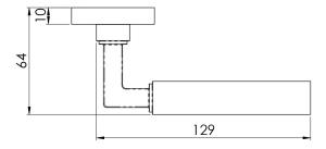
Lever on a concealed fix 2 part screw on round rose. A stylish round bar lever reflecting the attention to detail in this range. Comes with a 25 year mechanical guarantee and is Fire door rated. Suitable for domestic and commercial use.
