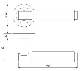
Lever on a concealed fix 2 part screw on round rose. A stylish knurled for grip round bar lever. Comes with a 25 year mechanical guarantee and is Fire door rated. Suitable for domestic and commercial use.
