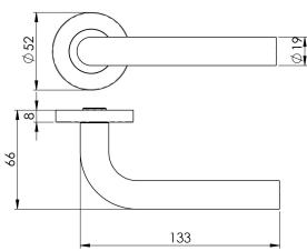
Lever on concealed fix press on round rose. Straight round bar lever which curves at the stem creating a smooth flowing line. Part of the Steelworx range in grade 304/201 Stainless Steel. Comes with a 10 year mechanical guarantee and is Fire Door Rated.
