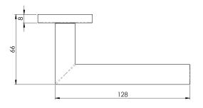
Lever on concealed fix press on round rose. Straight round bar lever neatly mitred where it adjoins the stem. Part of the Steelworx range in grade 201 Stainless Steel. Comes with a 10 year mechanical guarantee and is Fire Door Rated.
