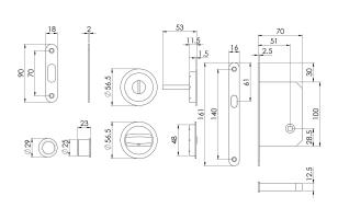
Sliding bathroom door set comprising of a turn and release, finger pull and a lock . The slim lock has a hook bolt which locates into a keep which is morticed into the frame. The thumb turn operates the lock mechanism. The flush fitting roses are sunk into the door and the coin release provides access in case of emergency.
