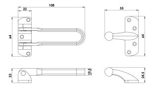
This door guard is a stronger alternative to the standard door chain and prevents a door from opening fully for added security. This easy to install guard allows the door to open to approximately 30-50mm for viewing (depending on fixing position) if without a door viewer. Supplied with fixings in matching finish.
