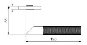
Lever on concealed fix threaded rose. A diamond pattern knurled round bar. Part of the Steelworx range in grade 304 Stainless Steel. Comes with a 10 year mechanical guarantee.
