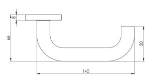
Lever on concealed fix press on round rose. Safety Lever, a 19mm round bar return to door lever. Ideal for public/office doors where a more ergonomic operation is a necessary requirement. Part of the Steelworx range in grade 201 Stainless Steel.
