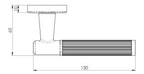
Lever on a concealed fix 2 part screw on round rose. The Image lines lever is a modern lined barrell sectional lever with a T-bar Stem. The chamfered edge concealed fix rose reflects the attention to detail in this range. Comes with a 10 year mechanical guarantee.
