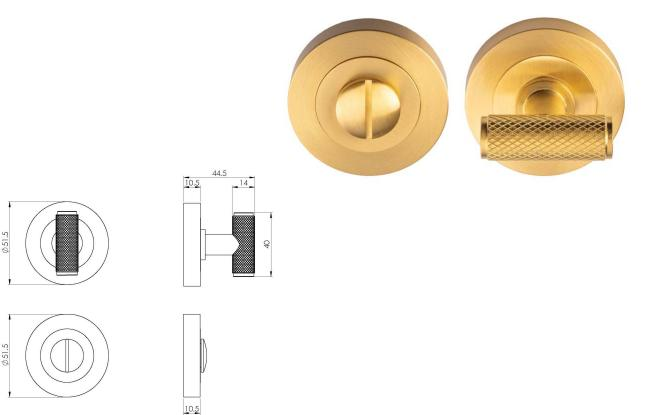
Thumbturn and release on a screw on rose, concealed fix. Designed to match the Syntax Lever on rose from the Manital collection. Supplied in a T-Bar design with a knurled bar, available in SB,MB,CP & SC.
