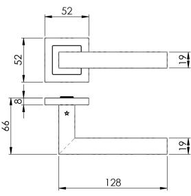
A square cut straight bar lever on a concealed fix square press on rose. An unfussy design which will blend well in a variety of applications. Part of a square themed designer lever collection in the Steelworx range in grade 304 Stainless Steel. Comes with a 10-year mechanical guarantee.
