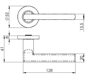
Lever on concealed fix press on round rose. A straight smooth round bar lever on rose. Part of the Steelworx Grade 304 stainless steel range. Comes with a 10 year mechanical guarantee and is Fire door rated.
